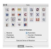
Note: In CFF-based OpenType fonts, the outermost contour is expected to be counter-clockwise. In glyf-based OpenType fonts, the outermost contour is expected to be clockwise. With both formats though, each contour needs to have the opposite direction than the contour in which it is located.
